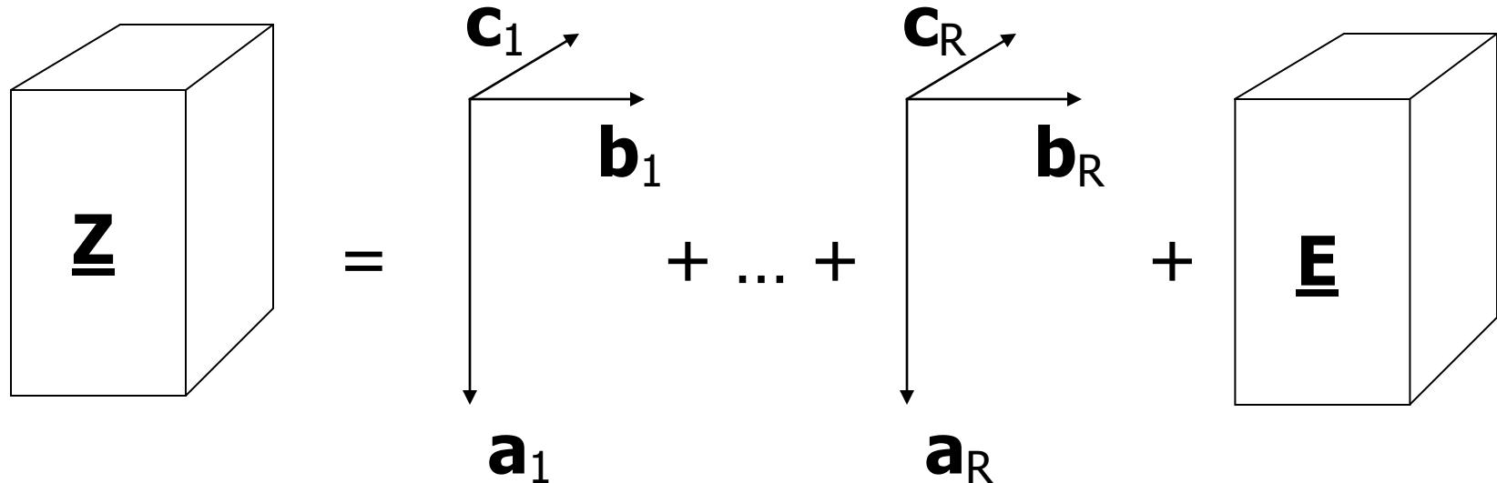
$$\underline{Z} = \mathbf{a}_1 \circ \mathbf{b}_1 \circ \mathbf{c}_1 + \dots + \mathbf{a}_R \circ \mathbf{b}_R \circ \mathbf{c}_R + \mathbf{E}$$
